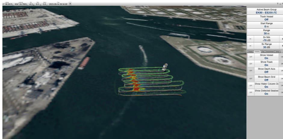
FIGURE 9 Drift of resuspended sediment to port of track behind a water injection dredge.
