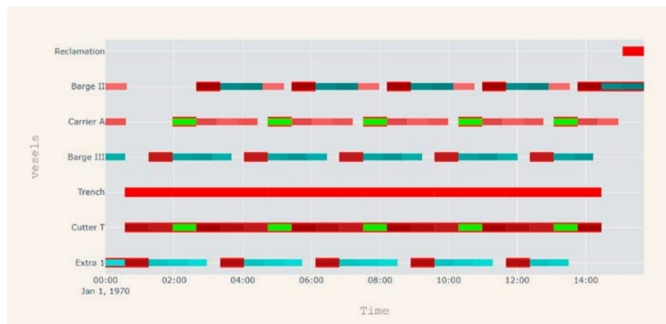
FIGURE 3 The Gantt chart of the loading and moving activities over time for the cutter and the barges. The critical path has been calculated and added to the plot as a red line under and over the relevant activities.
