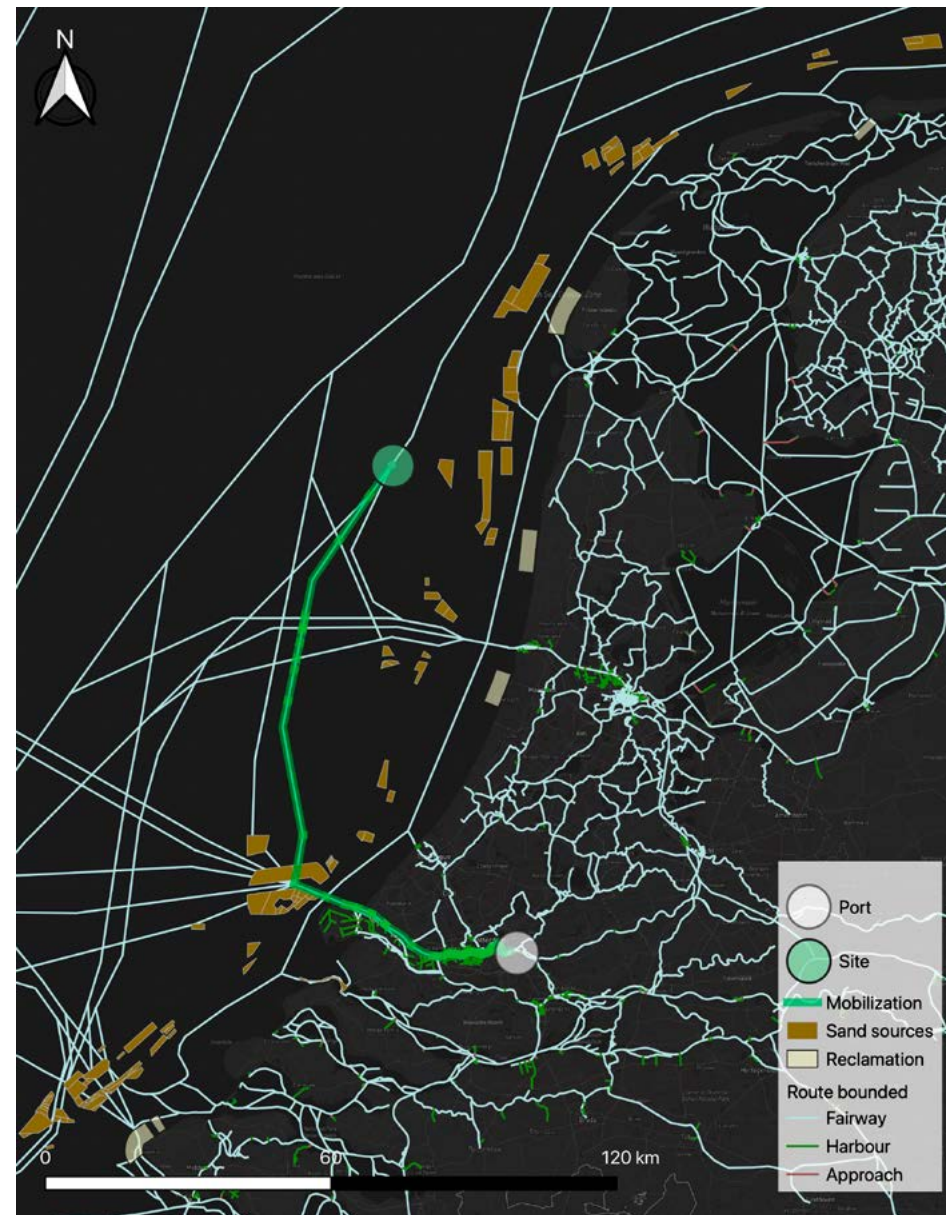
FIGURE 6 Example transport of a TSHD (green line) from an origin port (white dot) mobilised (green line) over the Dutch Fairway Network (light blue lines) to the trench (green dot) using an OpenCLSim routable. Brown patches are sand mining sites and yellow patches are beach nourishment locations.
