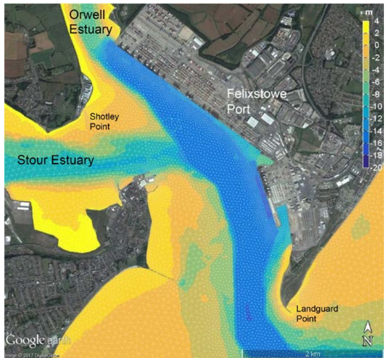
FIGURE 6 Model geometry and mesh within Harwich Harbour.
