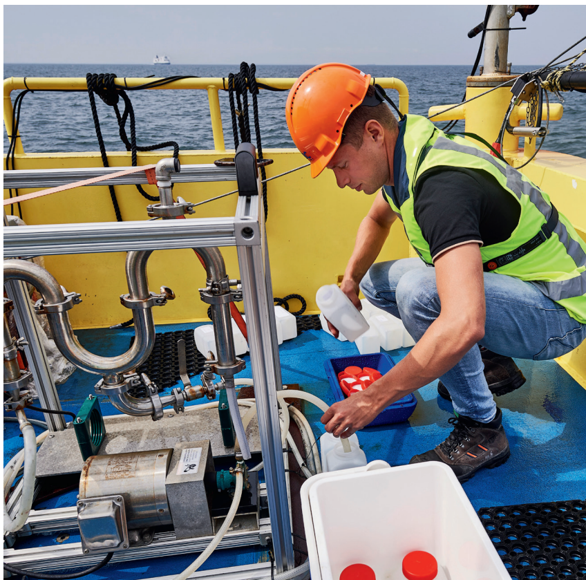
FIGURE 9 Spill engineer taking water samples for calibration and verification of instruments.
