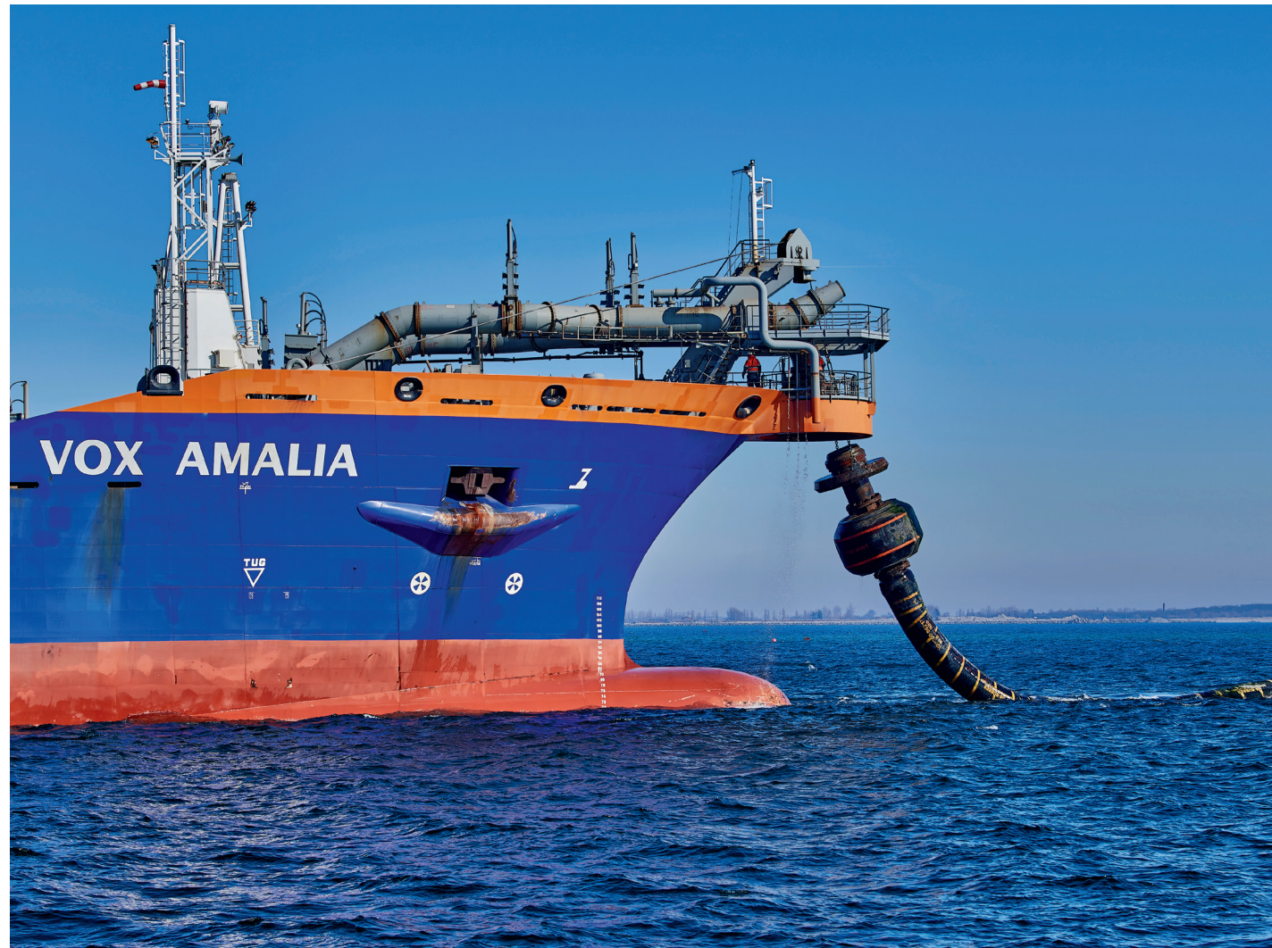
FIGURE 13 Trailing Suction Hopper Dredger, Vox Amalia.
