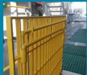
The hatch safety cover is a crew initiative that was built and installed on board Jan De Nul's trenching and offshore support vessel, Adhémar De Saint-Venant. Designed to increase safety on board, the cover ensures protection of the access ladder between decks. It prevents people falling through the opening and stops objects from falling down to lower decks.
