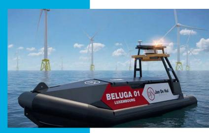
its mobility and seaworthiness for data acquisition under rough conditions. It is a user-friendly, cost-effective and low-risk platform for data acquisition at sea and serves as an alternative or addition to larger manned vessels.
