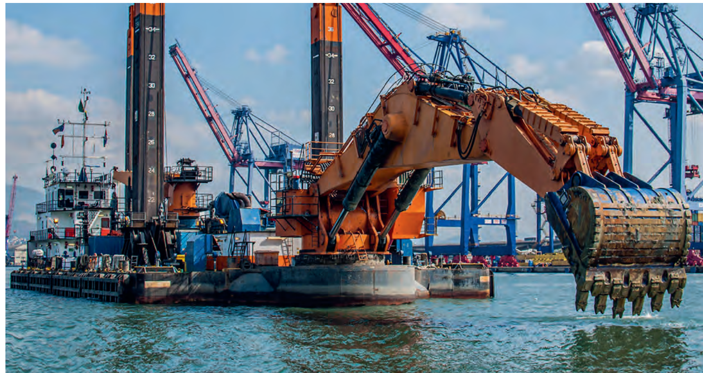
FIGURE 4 Van Oord's Goliath with Backacter 1100 excavator can be equipped with a 40 m 3 bucket. Photo © Van Oord.
