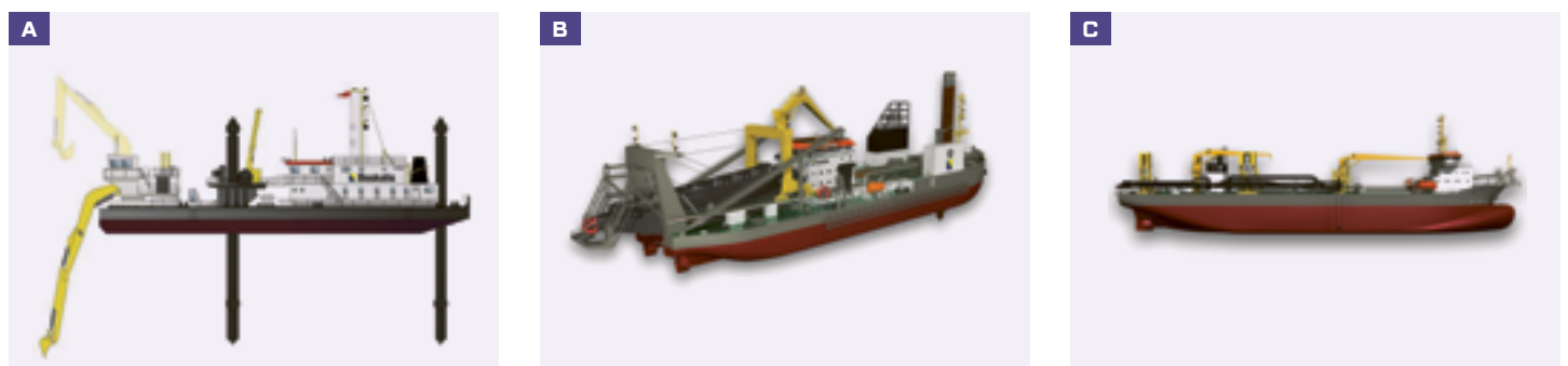
FIGURE 2 Different types of dredging equipment (source Boskalis, 2018). (A) Backhoe Dredger (BHD). (B) Cutter Suction Dredger (CSD). (C) Trailing Suction Hopper Dredger (TSHD).
