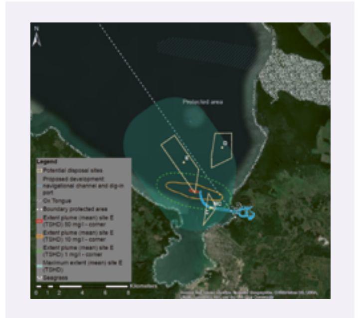
FIGURE 12 Extent of the sediment plume when disposing at the corner of disposal site E, based on the assumption that 5% of fines reach the far field, a current velocity of 0.2 m/s and a settling velocity of 0.08 mm/s.
