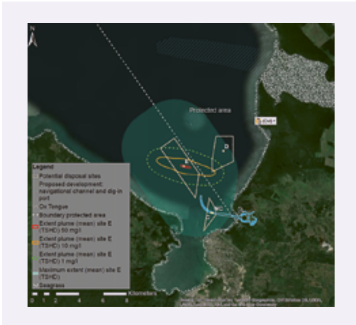
FIGURE 11 Extent plume disposal site E using TSHD.
