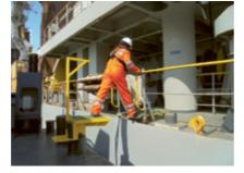
Jan De Nul's bollard step provides a solution that is both easy and quick to use, and is low on maintenance. Designed by crew, the bollard step transforms mooring equipment into a safe and secure step on which to make marine transfers.
