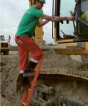
connection is possible. The benefit of the design is that you only need one type of ladder. DEME foresee one standard ladder with a maximum length that can be adjusted on smaller type of track excavators.
