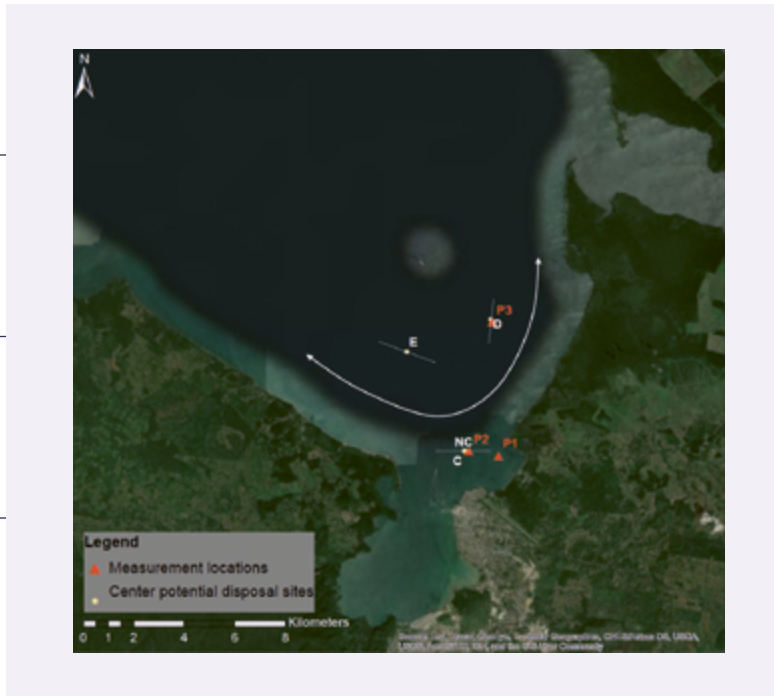
FIGURE 6 Schematisation of the measured current conditions as used in the plume dispersion study.
