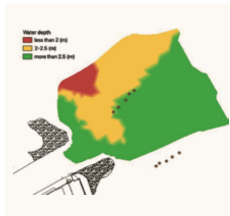
FIGURE 7 Colormap of water depth for specific ranges (more than 3.0 m, between 2.0–2.5 m and lower than 2.0 m) on 11 September 2020. The red circles indicates the GPS reference of the mooring points of inlet and outlet ejectors pipelines. The ejectors are installed between the inlet/outlet mooring points, as shown in Figure 2.
