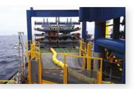
**FIGURE 14** The CPS rack can store up to 48 CPS systems, in different layers.
