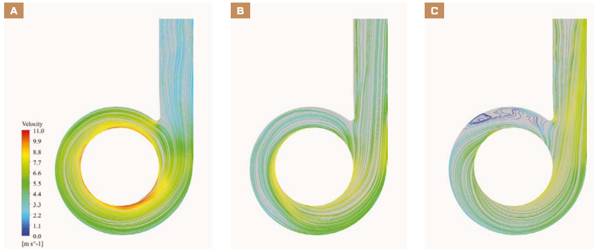
FIGURE 7 Instantaneous streamlines in the volute casing with water flow shown for three conditions: 0.5Q_d [A], 1.0Q_d [B] and 1.3Q_d [C].
