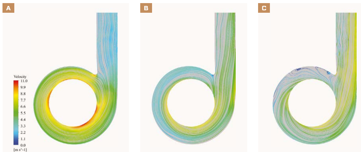
FIGURE 8 Instantaneous streamlines in the volute casing with silt-laden flow shown for three conditions: 0.5Q_d [A], 1.0Q_d [B] and 1.3Q_d [C].
