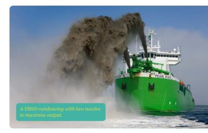
In contrast, one of the smallest TSHDs has a hopper capacity of only 3,400 m<sup>3</sup>, a deadweight of 4,800 tonne with a length of only 93.3 m and a loaded draught of 5.0 m. Her maximum dredging depth is 26.5 m with a suction pipe diameter of 800 mm, a trailing pump power of 1,250 kW and a power when pumping ashore of 2,000 kW, and a propulsion power 2 x 1,000 kW. Its total installed diesel power is 4,100 kW and she has a speed of 11.5 knots.
