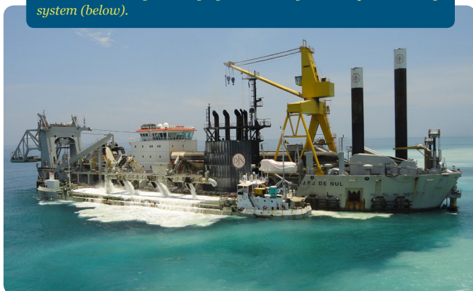
CSDs can discharge dredged material either via a floating pipeline to shore (above) or by discharging it into a barge with a special loading system (below).
