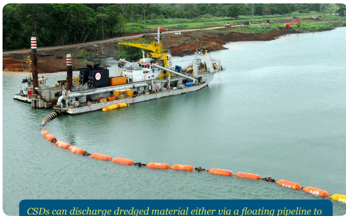
CSDs can discharge dredged material either via a floating pipeline to shore (above) or by discharging it into a barge with a special loading system (below).
