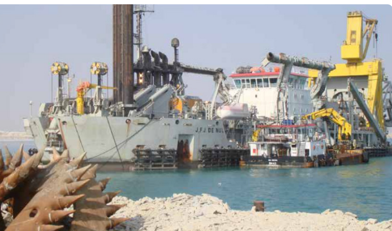
A CSD like this one from Jan De Nul is used for cutting sand, hard clay and rock.
