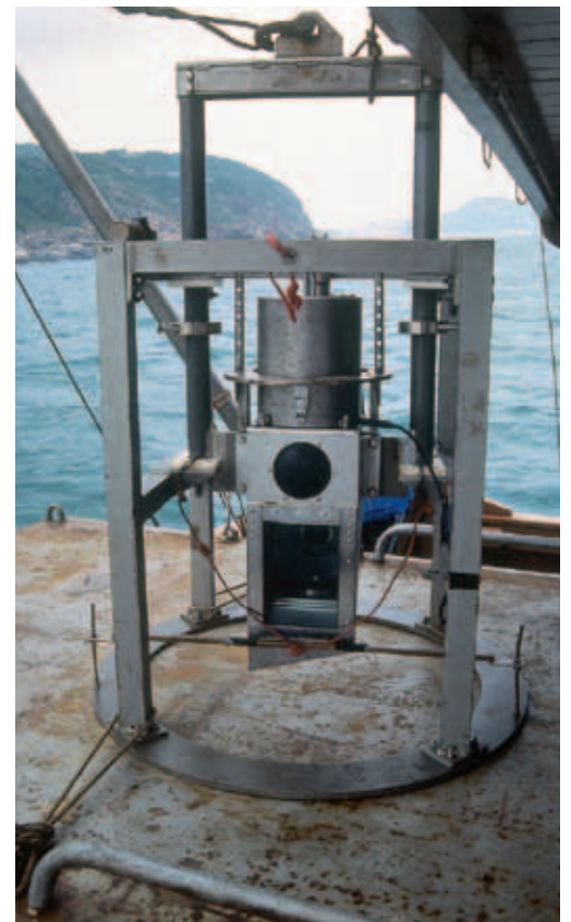
BELOW. This remote ecological monitoring of the seafloor (REMOTS) camera is another way of measuring the effects of dredging.
