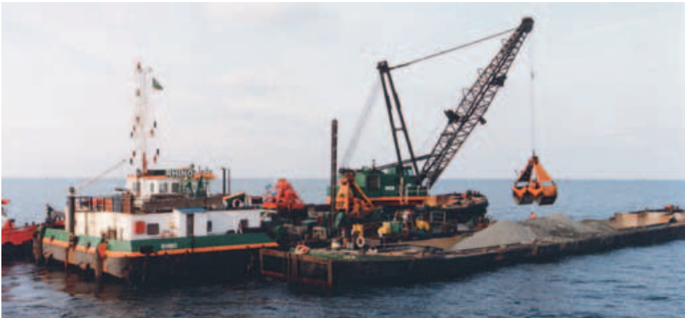
A grab or clamshell dredger mounted on a rotating cab.
