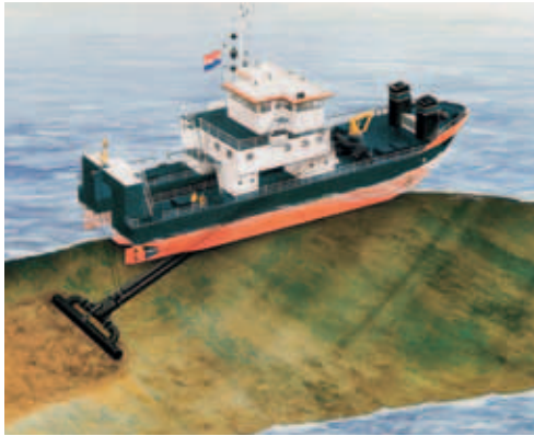
RIGHT. Artist's impression of water injection dredger at work.
