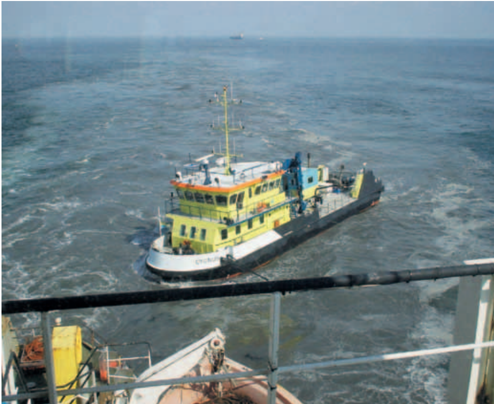
LEFT. Both large and small survey vessels are used to measure the dynamics of waterways such as current speeds, turbidity, temperature, salinity and suspended sediment levels amongst other parameters.
