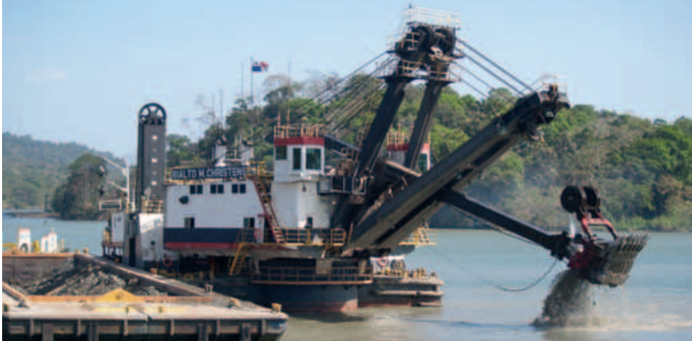
Dipper dredgers are particularly suited for dredging boulders and stiff clays.
