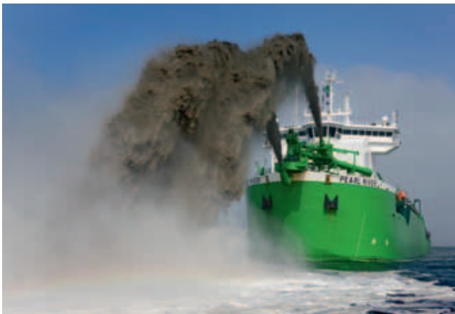
BELOW. A trailer placing sand by rainbowing with a double nozzle.
