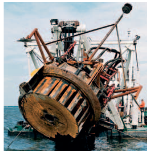
TOP. An encapsulated bucket dredger is an ecologically sound design for dredging contaminated sediments.
