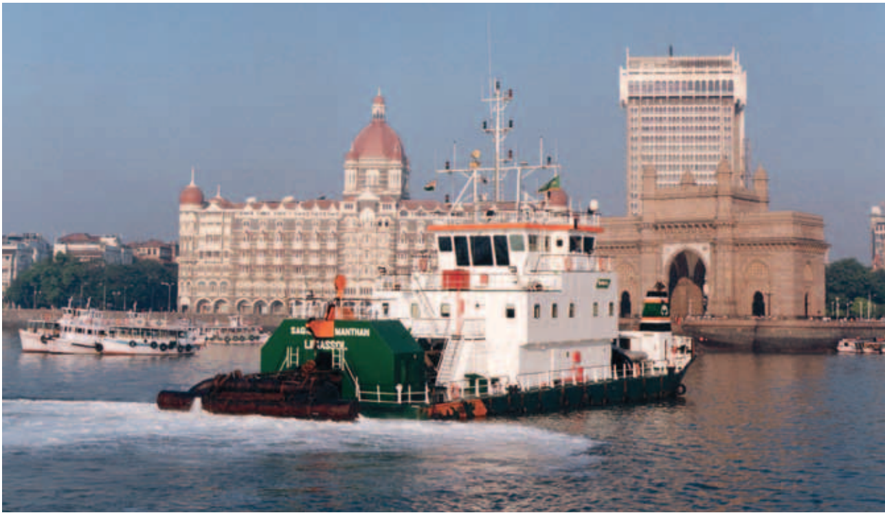
ABOVE. A water injection dredger was a cost-effective way to level the seabed in Mumbai, India.
