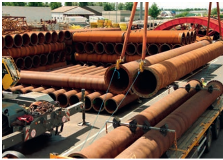
Figure 8. Made of low-density polyethylene (LDPE), Dhatec's System88 cradles stack and hold pipes in a two-by-two configuration.
