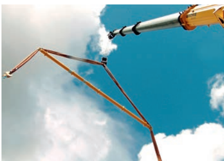
Figure 5. A modular spreader separates the soft slings – ensuring they are always ready to lift – as well as lightening the overall weight for riggers.
