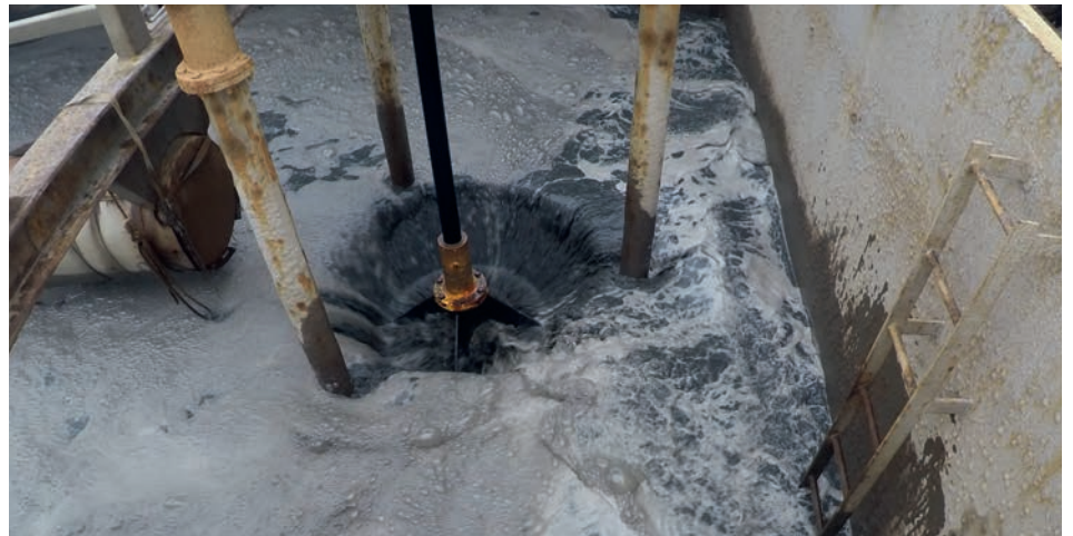
Figure 10. Overflow in a typical dredging vessel shows the turbulent flow with air inclusion.
