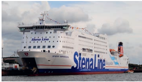
Figure 3. The Stena Germanica was converted to Methanol under Lloyds Register classification in 2015.
