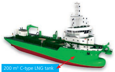
Figure 7. Royal IHC's hull and bulb design which reduces wave and fuel consumption.
