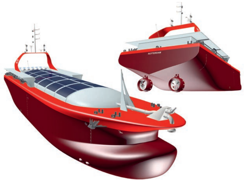
Figure 16. A 3D impression of the 2050 concept shows the unmanned vessel with fuel cell drive and hub-less propellers.
