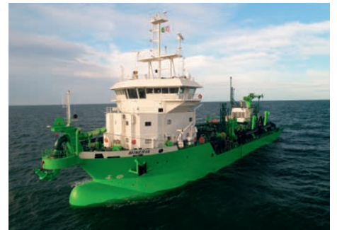
Figure 8. The Minerva is the first TSHD sailing on LNG in the world.
