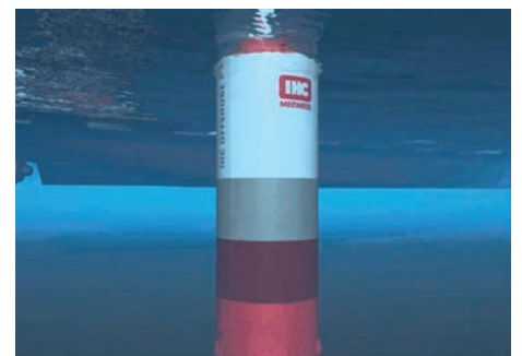
Figure 11. The 'IHC Hydrohammer' is a pile driving installation with reduced noise levels to allow for pile driving even in the more sensitive areas.
