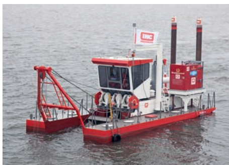
Figure 9. Test with a PEM fuel cell as auxiliary power – which uses hydrogen – during sea trial of a Beaver 40.
