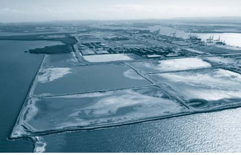
Figure 3. Aerial view of Fisherman Islands, looking back towards the city of Brisbane. In the foreground, the current reclamation area is divided into paddocks, where dredged material is pumped to reclaim land.
