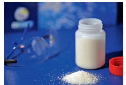
Figure 2. Polymers are commercially available in many forms including emulsion (left) and powder (right).
