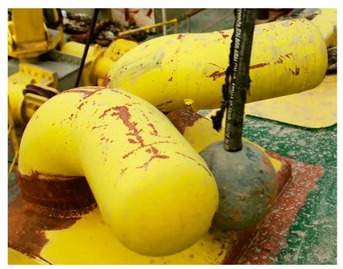
Figure 2. A V-shaped mooring bollard
