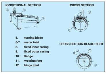
Figure 1. The scoop-head (general lay-out).
