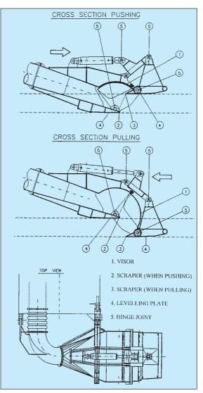
Figure 3. The sweep-head (general lay-out).
