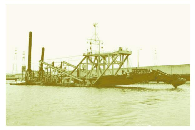
A buffer system is planned just behind the dredge. This makes it possible to slow down the suction (dredging) process without interrupting the reclaiming process. In this way the buffer system will prevent water from having to be pumped to clean the dredge pipes before stopping the dredge process.
