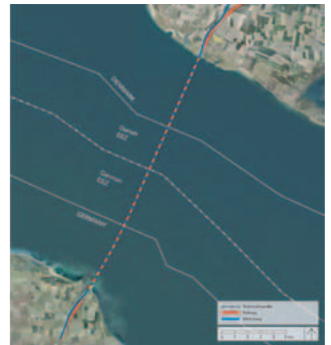
Figure 1. Conceptual Design alignment (road shown in blue and rail shown in red).
