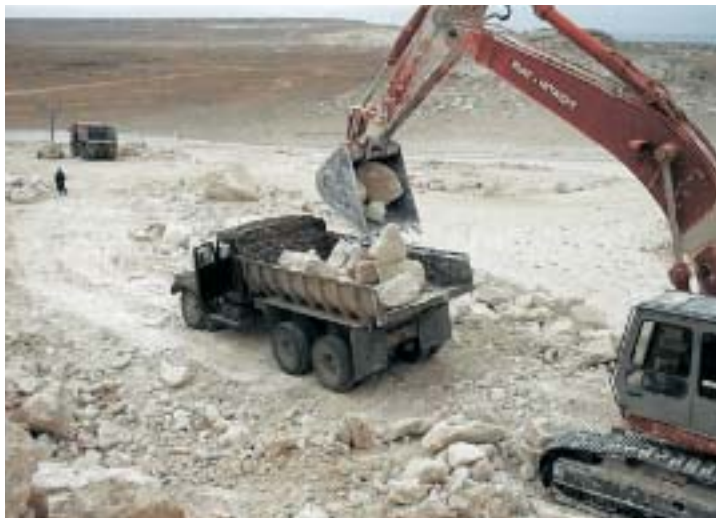
Figure 7. The rock from the local quarry was an alluvial deposit of limestone and more porous than originally thought, so a new quarry was developed.
