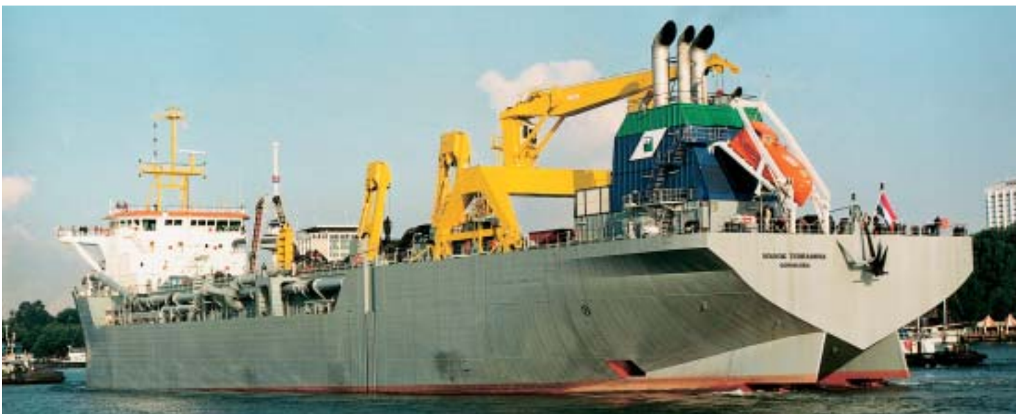
Figure 15. Hull design of the Jumbos: twin gondola escutcheon stern, without propeller shaft struts.
