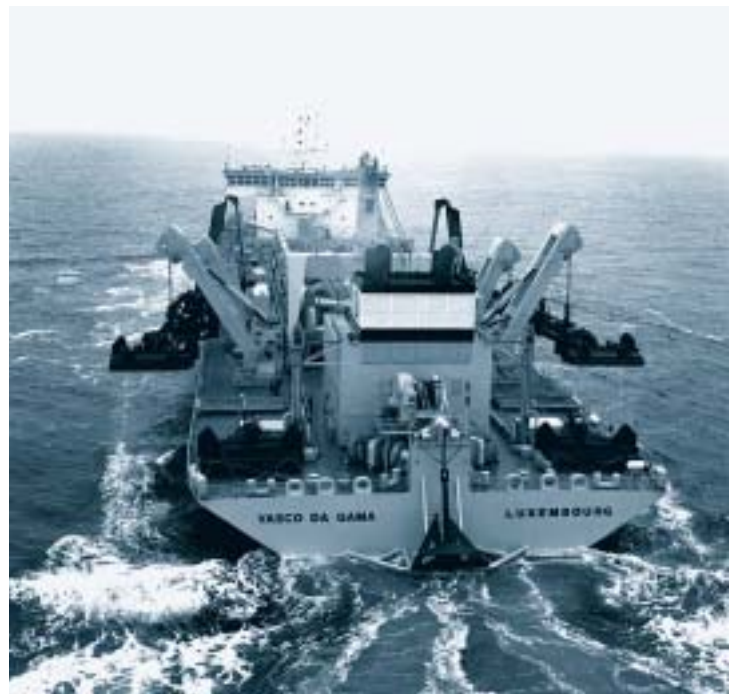
Figure 11. Queen of the Netherlands (23,347 m 3 ), launched in 1998, was part of the wave of jumbos built in the late 1990s. (Photo First)
