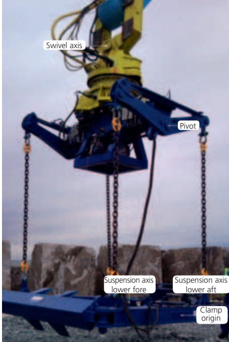
Figure 12. Left: The swivel axis below the end of the stick, pivot axis and taut wire system. The taut wire system measures by means of a wire the distance and angular offset to the block clamp from a fixed point located below the swivel. Above: Block clamp suspended by chains.
