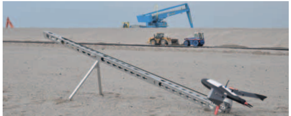
Figure 26. The Gatewing X100 ready for takeoff.
