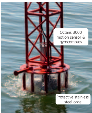
Figure 14. Protective stainless steel cage with on top the Octans 3000 subsea gyrocompass and motion sensor.
