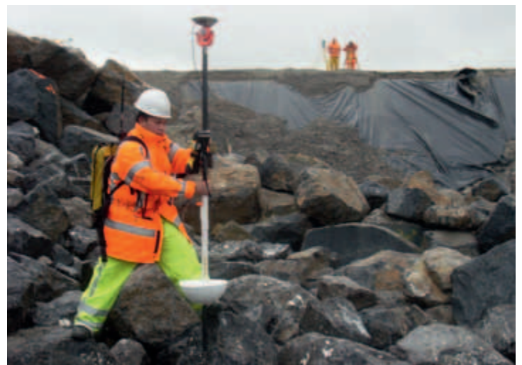
Figure 6. Measurement with semi-spherical foot and point measurement carried out on 150-800 kg rock grade.
