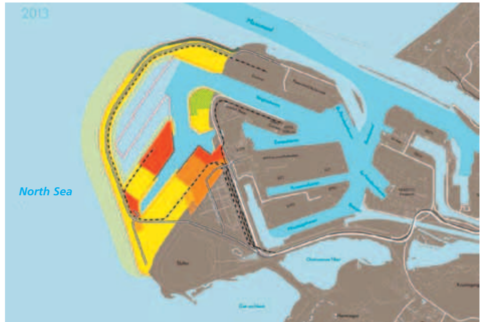
Figure 1. Sea defence, harbour basins and 700 hectares of new port area (Phase 1, in yellow). Grey area indicates Maasvlakte 1).
