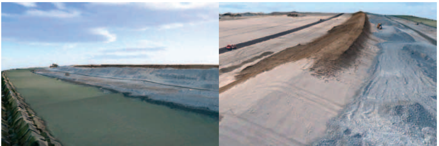
Figure 27. Two views of the Gatewing X100 results displayed with Autodesk Infrastructure Modeler. Left: Part of the block dam and stony dune. Right: The stony dune with sand core and clay protection.
