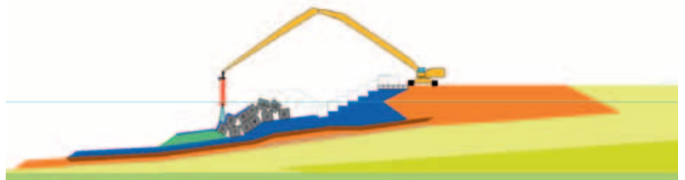
Figure 19. Multibeam survey on the 1-10 tonne toe structure and the second layer of blocks below the waterline.
