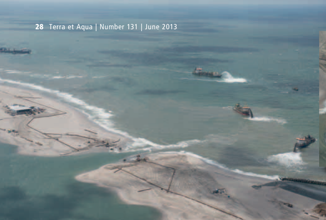
Figure 28. Closure of the soft sea defence on July 11, 2012. TSHDs from far left to right: Vox Maxima , Prins der Nederlanden , Crestway and Ham 317 . Insert: Closing the gap, the land-based equipment spreading sand.
