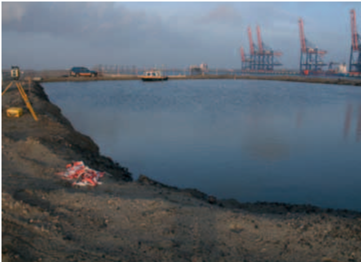
Figure 7. Survey vessel Seapilot in the background carrying out a survey in the test pit. The Trimble SPS 930 Robotic total station was used to monitor possible variances in RTK height onboard the survey vessel.
