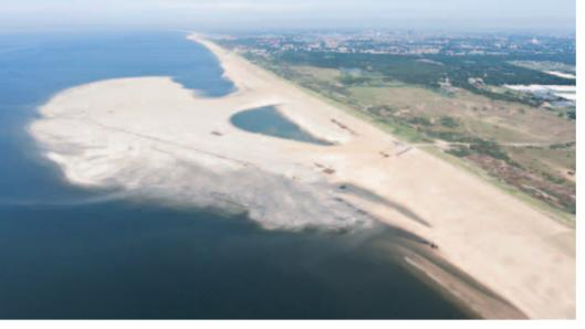
Figure 5. Delfland Sand Engine on June 14, 2011 showing the progress of construction of the peninsula which will extend about 1 km into the North Sea.
