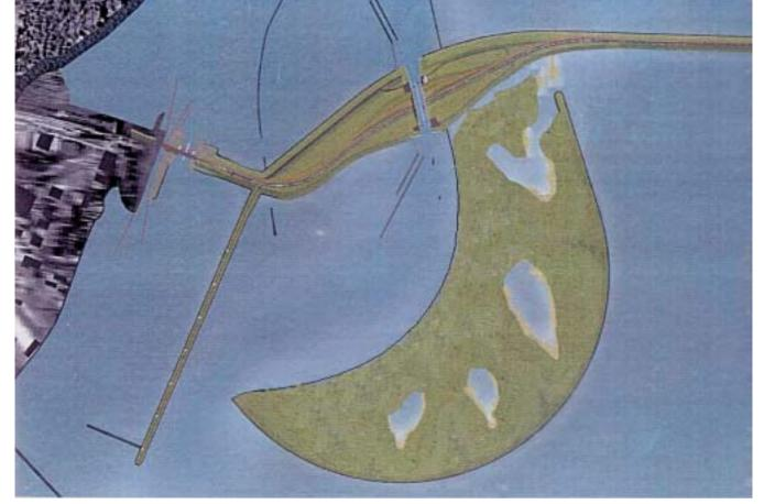
Figure 1. Helicopter view of the Enkhuizen Naviduct with the pre-shore areas: The geotubes are worked into the dams.
