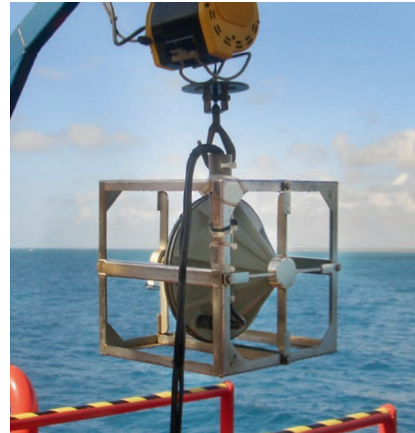
Figure 7. FaunaGuard transducers and hydrophone in São Francisco do Sul, Brazil.
