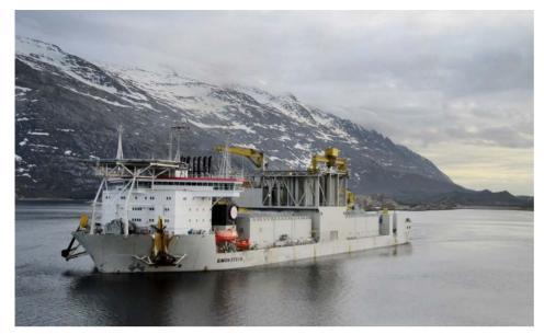
Figure 6. A fallpipe vessel (FVP) being used for subsea rock installation in Norway. Dredging vessels come in a variety of types which may require different fuel solutions.
