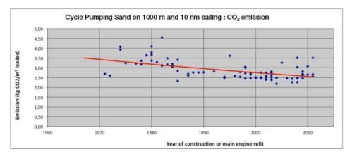
Figure 3. Efficiency improvement for Trailing Suction Hopper Dredgers.
