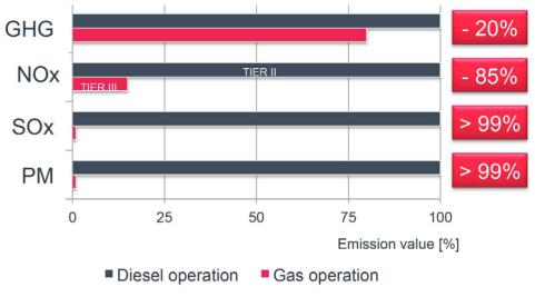
Figure 4. Air Emissions Reduction, Gas vs Diesel operations. Gas mode offers IMO compliant operation without any additional after treatment technology.
