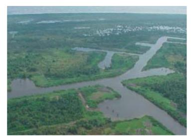
Figure 6. Hydrologic modification — notice the dredged material canal banks and the oil wellheads.
