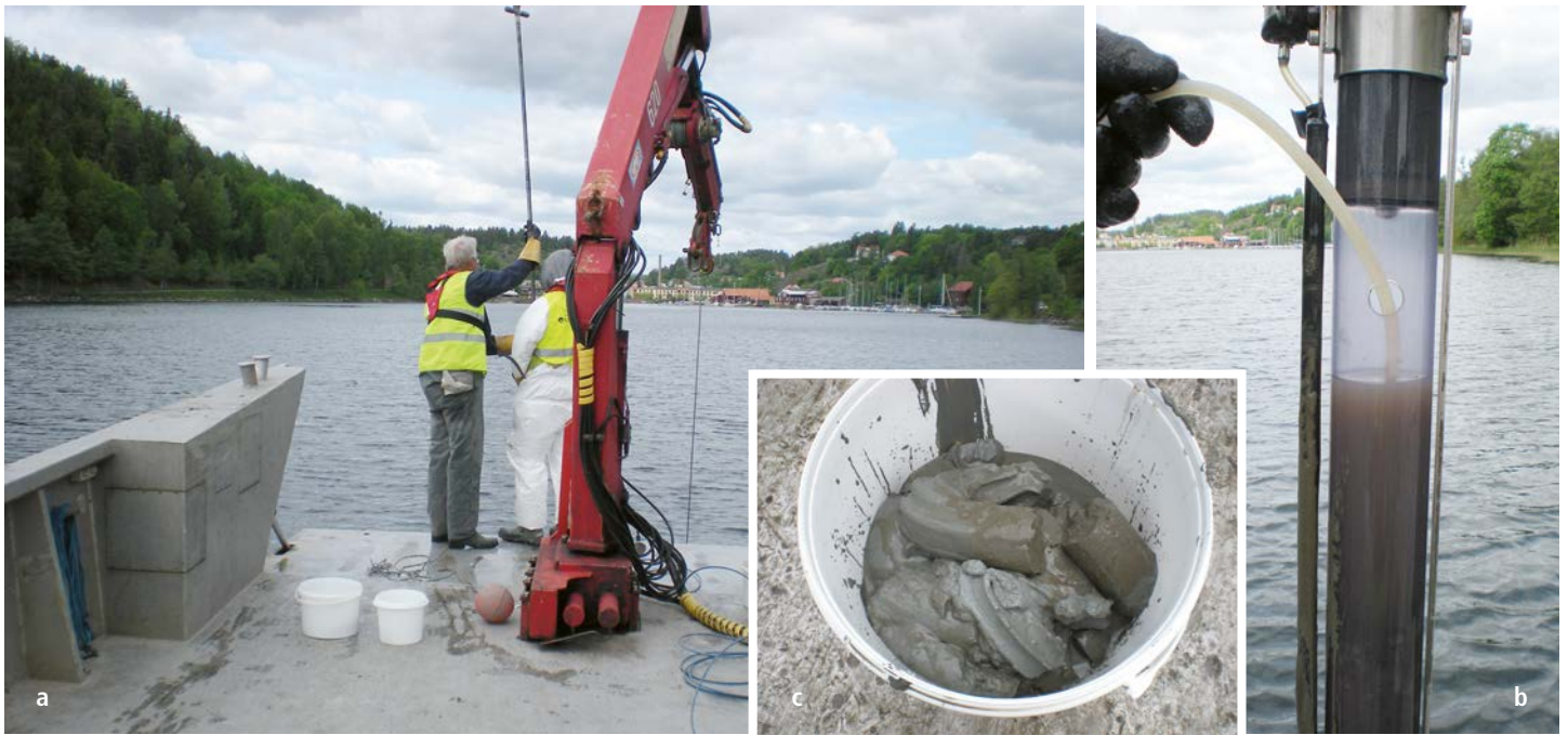
Figure 5. (a). Sediment sampling performed in the Valdemarsviken fjord (b). A manual core sampler collecting sediment sample. (c). A view of the collected sample.
