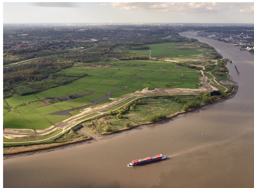
Left, Figure 5. Before: Aerial photograph of the northern part of the project site along the River Scheldt shows the situation with agricultural land before the start of the project. This part is being converted into a tidal marsh by the creation of a Flood Control Area with a Controlled Reduced Tide (FCA-CRT) (see Zone 4 in Figure 3B and Figure 4 for more details about the FCA-CRT concept). Right, Figure 6. After: Aerial photograph of the southern part of the project site along the River Scheldt: wetland as bird area (Zone 1 in Figure 3B) and alder brook forest (Zone 2 in Figure 3B).
