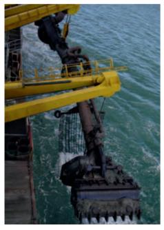
Figure 10. Turtle deflector installed on the drag head of the TSHD.
