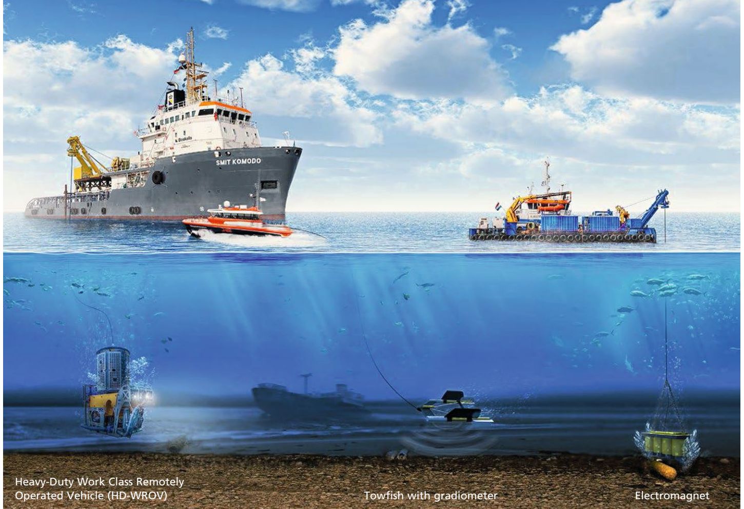
Figure 3. Left, a Heavy-Duty Work Class Remotely Operated Vehicle (HD-WROV) used to locate and salvage ammunition. Middle, a towfish with gradiometer to locate ammunition. Right, an electromagnet for salvaging ammunition.
