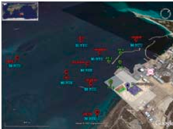
Figure 11. To protect the indigenous sea grass, turbidity monitoring took place at 12 strategic points.
