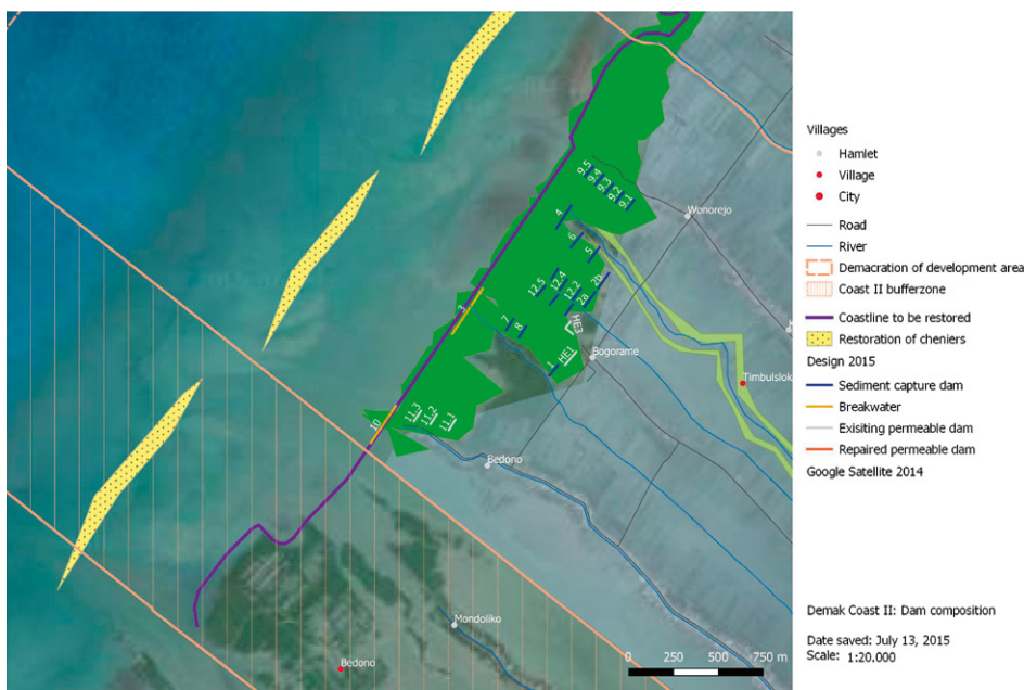
Figure 5. Permeable dam layout (to be) constructed in 2015 and 2016 in the Demak district with a sketch of the final configuration.
