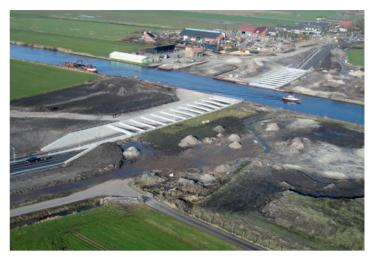
Figure 8. Aerial view of the Frisian Lakes Project: The new roadway goes under the canal which improves traffic flow.
