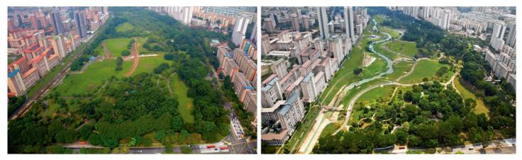
Figure 26. Singapore's Kallang River before (left) and after (right) Aquapuncture was applied. The concrete canal was changed into a meandering river, bordered by green parks on each side.
