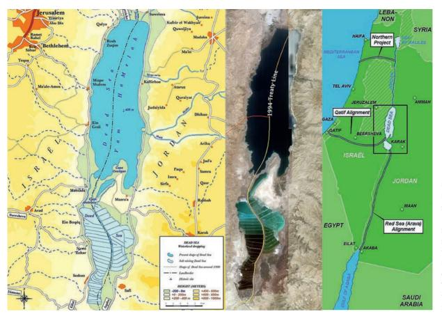
Figure 22. Map of the Dead Sea indicating shorelines now and in 1900 and a satellite photo. Right, the three pipelines connecting the Mediterranean, the Dead Sea and the Gulf of Aqaba and Red Sea. The choice was made for the Red Sea-Dead Sea Connection.
