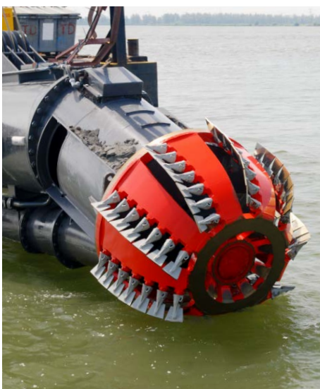
Figure 11. Lancelot cutter increases production, and thus lowers energy use per cubic metre dredged material.
