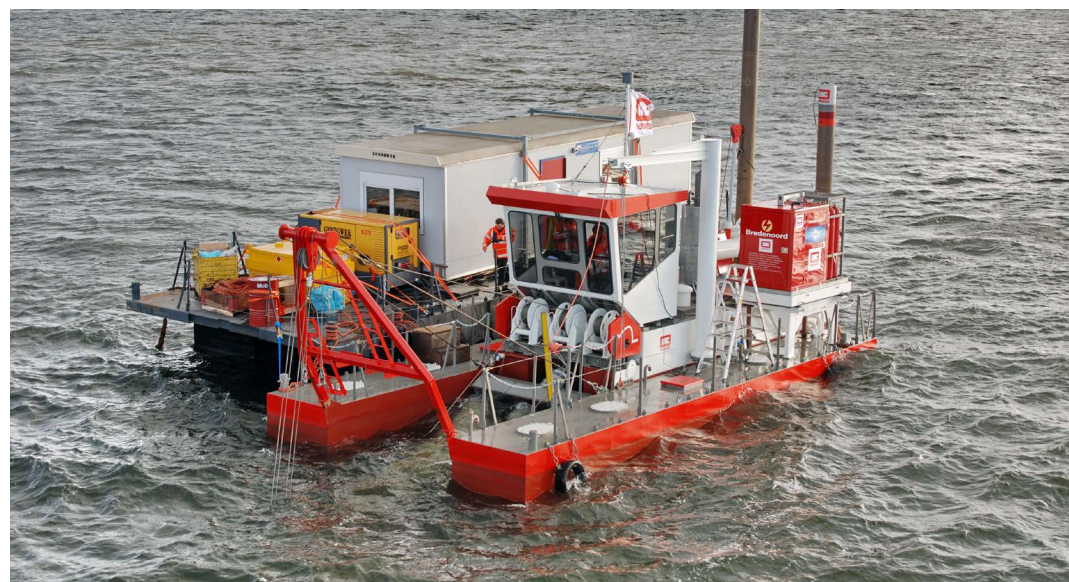
Figure 12. Testing Hydrogen as auxiliary fuel supply during the trial of the IHC Beaver 40.
