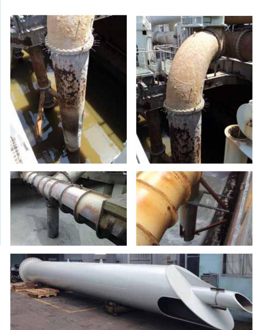
Figure 5. Top photos, installed deep load systems; below, a newly fabricated extended discharge pipe for a TSHD.
