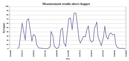
Figure 9. A measurement graph from on board a hopper dredger. The typical work rhythm can be identified: high peaks (going up to 100 ppm) during filling hopper and the obvious decrease of H<sub>2</sub>S measured during sailing.
