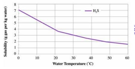
Figure 1. This graph shows the solvability of H<sub>2</sub>S gas in water.
