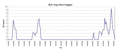
Figure 10. Reading on board a split barge, during the loading process with a cutter dredger. Again, the work rhythm can be identified (minor H<sub>2</sub>S peaks during loading barge).
